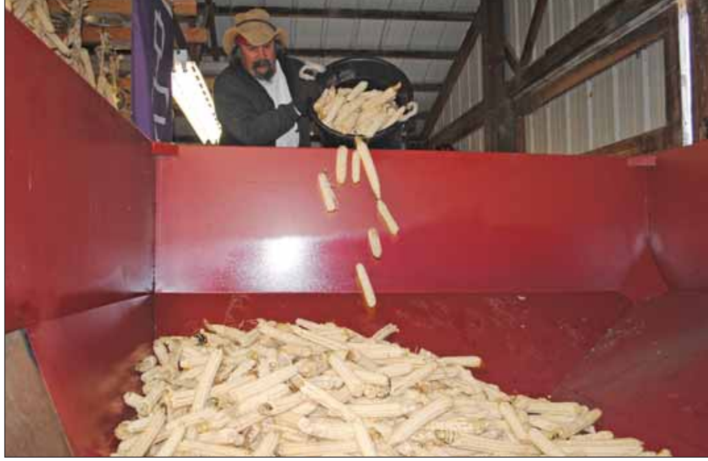
Submitted photo Jonesy Miller, Agricultural Worker, throws a bushel of corn in tsyunhéhkwá's new corn drying system. The new system dries corn in 30 days and prevents corn-loss to mold.
